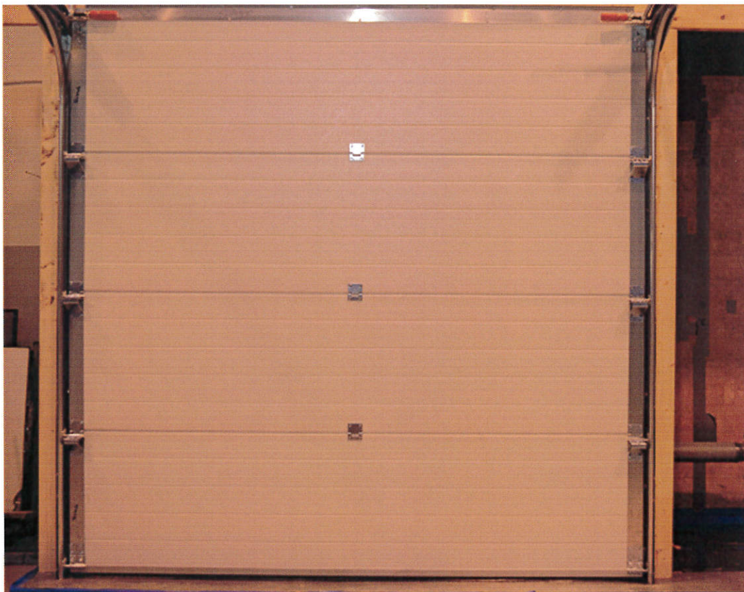
Figure 2. Tested door, DOCO SFR/SF/SRR garage door with Tecsedo panels, mounted in the test rig, as seen from inside.
